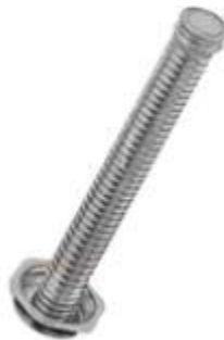
Figure 8 Blitz style pour spout. Note the male threads and the screen on end of spout. This spout is too large for unleaded fueled vehicles. The male threads will also fit the USGI plastic MFC jerry can. Just barely visible is the black rubber gasket.
