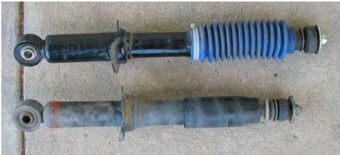
Tough Country Tacoma Shock (Top) with ball joint lower mount and Stock 4Runner Shock Bottom
