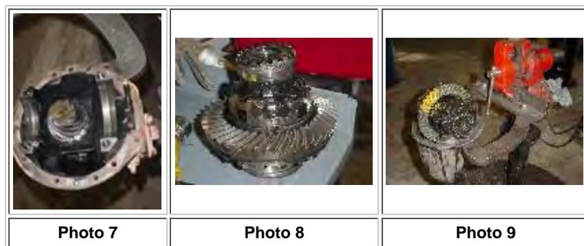
Photo 7: Rear differential with ring gear and carrier removed. Fork for the electric locker can be seen. The electric locker is gear driven and it is very important that the fork is lined up and properly timed. Stock pinion still in differential.
