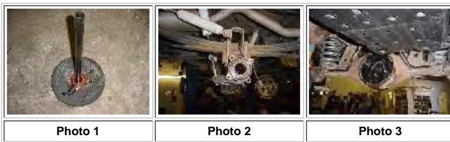
Photo 1: Rear axle removed from the rear axle housing.
