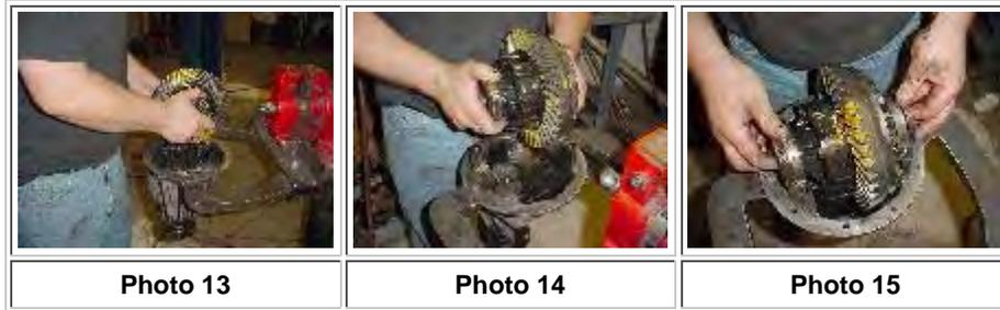
**Photo 13, 14 & 15: Setting the carrier back in the differential housing and aligning the adjusters.**
