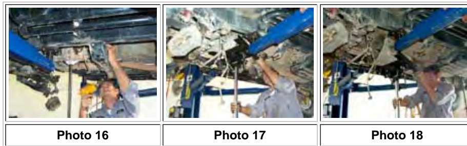
Photo 16: Pulling the 2WD Transmission.
