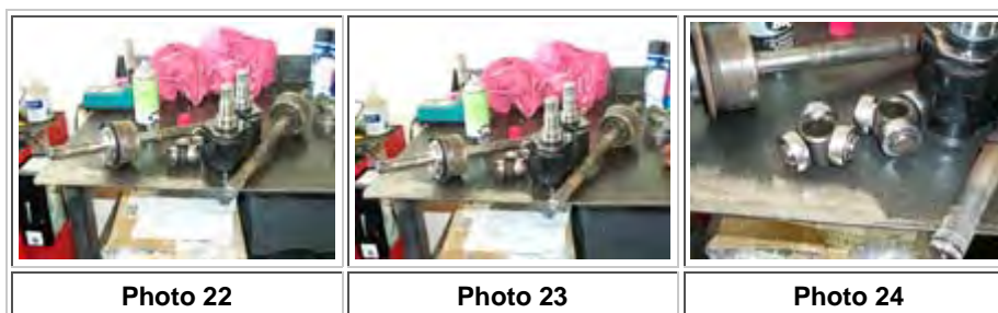
Photo 22: Rebuilding the manual hub Tacoma axles.
