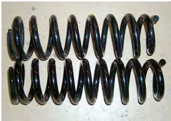
1998 Coil on top, 1999 Coil on the bottom. Both are from V6, 4WD and 16" wheel trucks. You can see the 1999 coil has 9 winds and the 1998 coil has 8.
