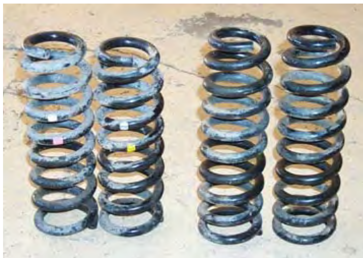
Here you can see the difference in height in the 8 wrap 2001 coils and the 9 wrap 1999 coils.
