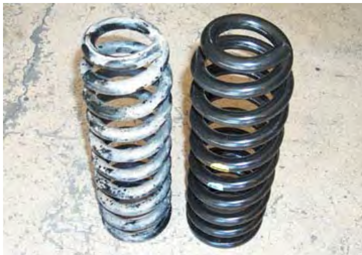
1999 4Runner coil left and Tundra TRD 4WD coil right. The two coils are the same height but the Tundra coil has a thicker wire.
