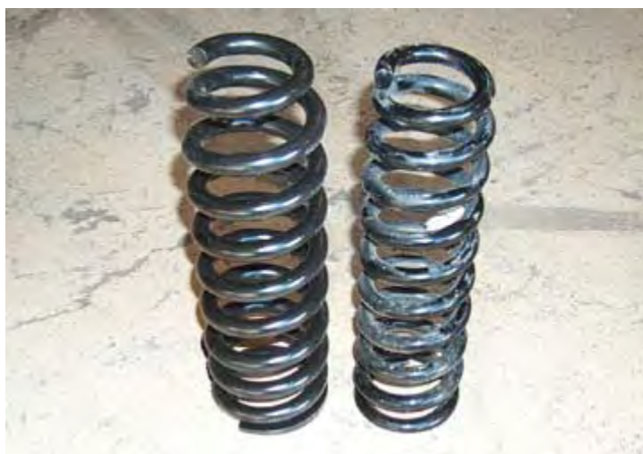
Tundra coil on the left and Old Man Emu 881 on the right. You can see they are the same height but the Tundra coil has a thicker wire.
