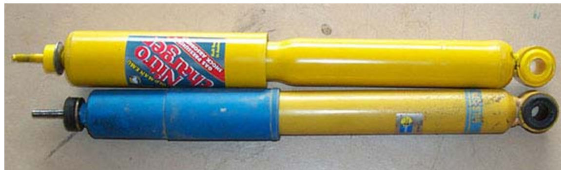
Stock 4Runner rear shock and Bilstein BE5-2451 rear shock.
